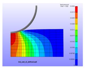
**Figure 2:** FE Model of biphasic cartilage indentation.
